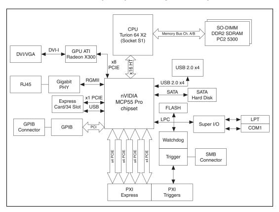
Figure 1-1. NI PXIe-8130 Block Diagram
